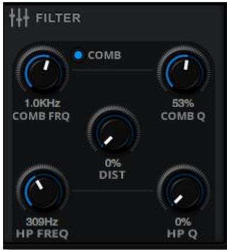
If you wish to do so you can apply distortion and filter effects to the reversed audio. RP-Reverse has a Distortion unit and a 12dB Low Pass and High Pass Filter. The Low Pass Filter can also be used as a Comb Filter.
